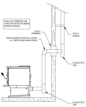
Figure 10 Basement installation
